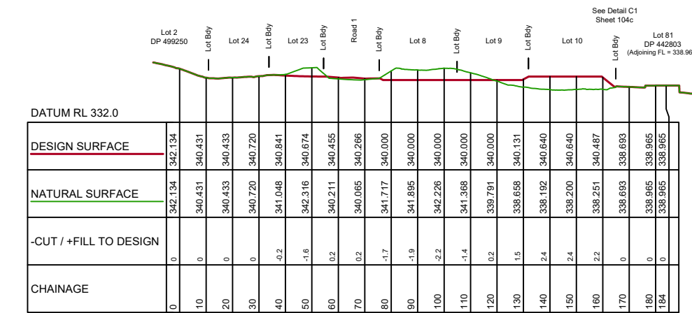
BULK EARTHWORKS - Earthworks Cross Section C-C
